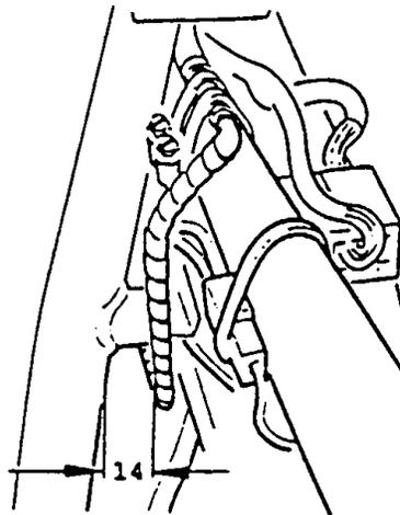
6. To prevent corrosion, any scuff marks on the fuel tank must be touched up. Our analysis of this chafing has proven that the fuel tank is only chafed a small amount. Therefore, it is not necessary to replace the fuel tank.
