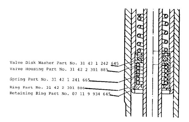
To install the two-part damper housing, use special tools No. 88 88 6 314 690 (clamp) and 88 88 6 314 693 (adaptor press). Fix the clamp and adaptor press as shown in the drawing below.
