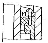
Note that this chamfer is always installed towards the perforated disk. Whenever repairs are performed, make sure both fork dampers are equipped with this new spring-loaded valve housing.
