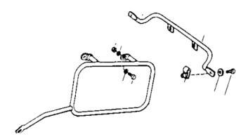
R100GS: If your customer chooses to install saddlebag mounts, the new cross support must also be installed.
